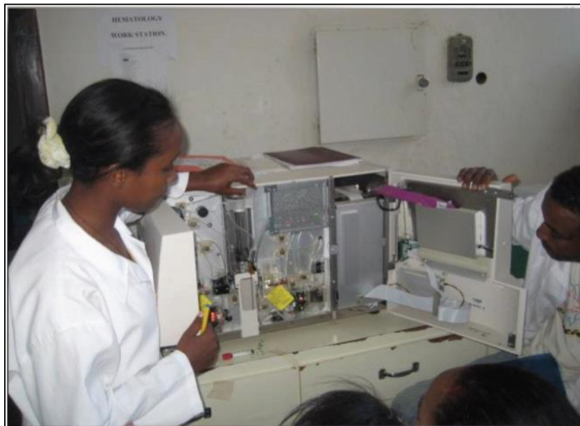
Training of lab techs on preventive maintenance of ART monitoring equipment (CD4 counter.)
